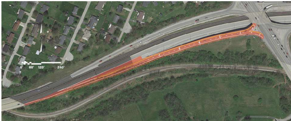
Concept sketch to extend EB ramp to US 60, adding striping to distinguish lanes.
