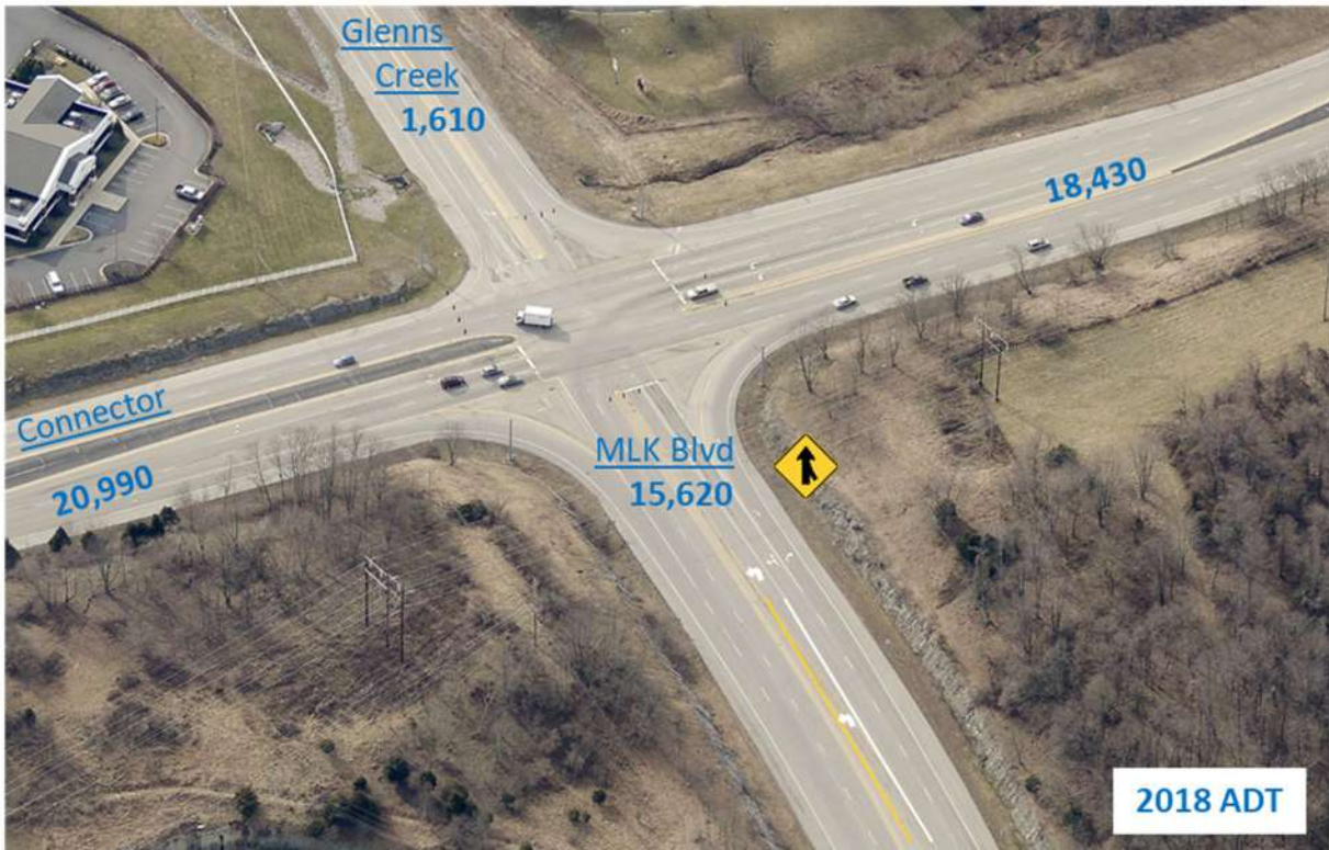
View south at KY 676 intersection with KY 1659, highlighting ADTs and proposed improvements.
