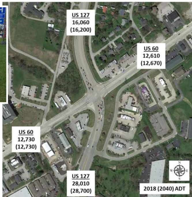
View east towards intersection (left). Existing and future ADT (right).
